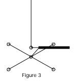
operation on 80/75 meters as well, but it is probable that at least one resonant radial will be required for low SWR on that band. It's important to note that cutting each conductor of rotator cable to a specific frequency will not work unless you separate it, angling each conductor away for most of its length because the longer ones will detune the shorter ones.
