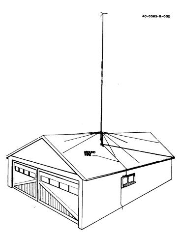
Figure 6 Completed Installation of 14AVO/WB-S
