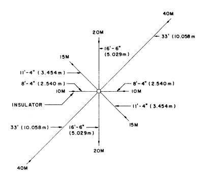
NOTE: RADIAL DIMENSIONS MEASURED FROM BASE TO INSULATOR.
